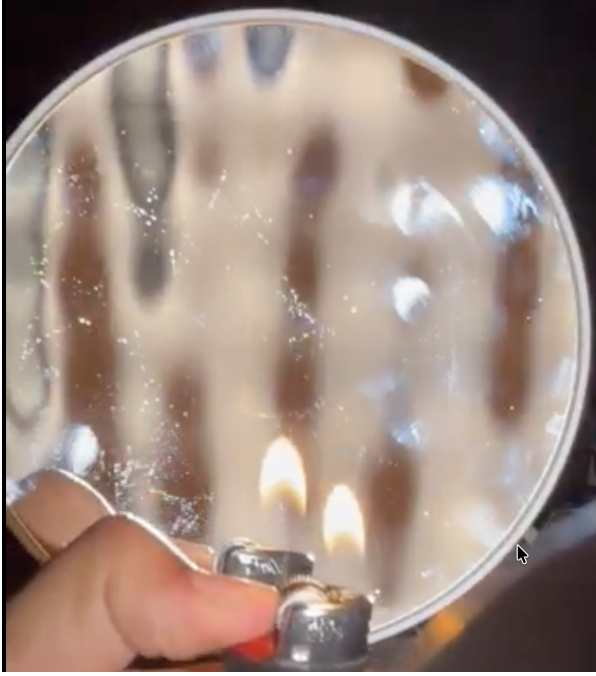
(a) Concave mirror used in the system ( f = 37 cm).
