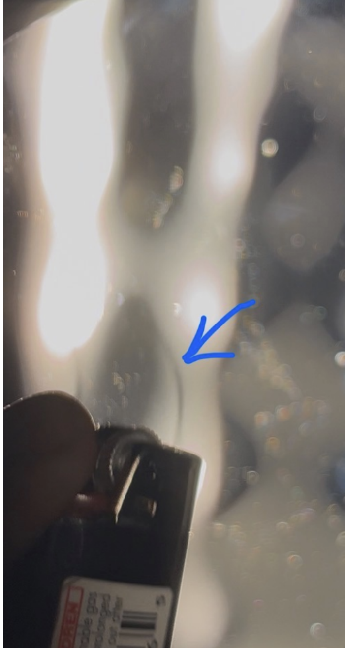
Figure 3: Schlieren visualization of lighter-induced convection. The observed bright and dark streaks correspond to spatial gradients in refractive index, revealing upward-moving thermal plumes and turbulent flow structures above the lighter.
